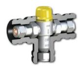
The tempering valves built onto the DH Hydronic hot water heaterscome preset at 50°C, but can be set at between 40°C and 55°C by removing the yellow cap and rotating the brass bolt beneath it.
