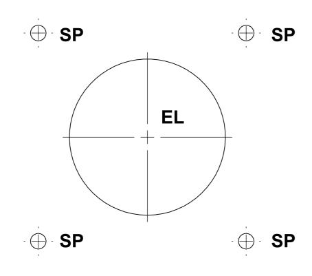
FS = FIXING SCREWS EL = EXHAUST CENTRE SP = SILICON PLATE HOLES
