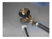
The breather tube fits onto the straw and is clamped down with an ear clamp.
